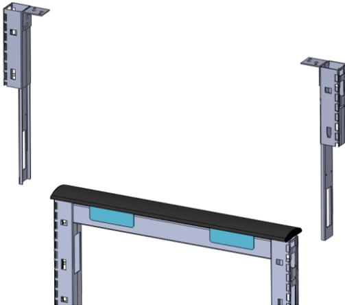
2. To remove the base frame top cap.
